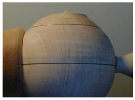
Next a matching cut will be made from left to right. Repeated cuts from will remove the material down to the ball. Watch the solid outline of the ball and cut away the fizzy image produced by the air and wood outside of the sphere. Once you have cut to the line or very close to it, remove the gouge ridges with light scraping cuts.
