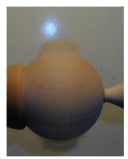
The ball's outline can be seen when the ball is spinning. A white background can make it easier to see. When first mounted in the cup the long grain of the wood will be perpendicular to the lathe ways.
